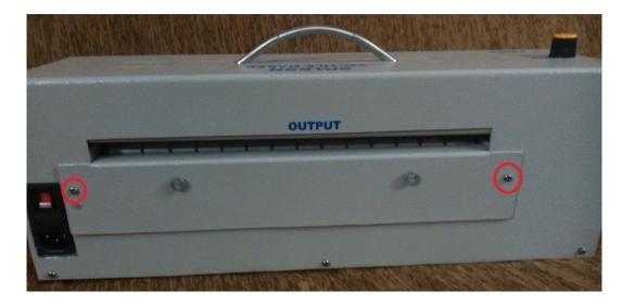
• Now place your thumbs on the metal spring clips at each side of the opening and push in (towards the machine sides) on the clips until they release the transport mechanism which will drop down. The paper can be removed. Reverse the above procedure to return the machine to working order. Ensure the transport mechanism clips firmly back into position.
